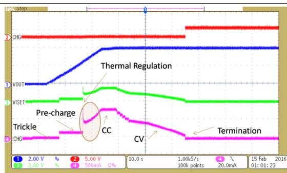
The IC temperature rises to 125°C and enters thermal regulation. Charge current is reduced to regulate the IC at 125°C. VIN is reduced, the IC temperature drops, the charge current returns to the programmed value
