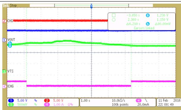
图 14. TS Entering and Leaving Cold Temperature
