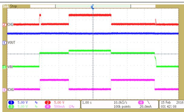
图 16. OVP From Normal Power-Up Operation –  $V_{IN} 0V \rightarrow 6V \rightarrow 7V \rightarrow 6V \rightarrow 0V$
